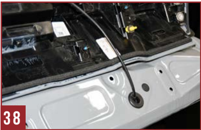
FIG. 38-39 Push the cable grommet into the sealing grommet position.
