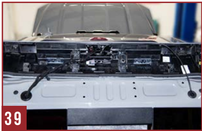
FIG. 38-39 Push the cable grommet into the sealing grommet position.
