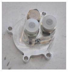
WARNING: When installing the Half Kit adapter, make sure the step on the bottom of the adapter is placed on the filter housing drain. Once the adapter is resting on the housing <u>DO NOT SPIN OR TWIST IT.</u> If the filter housing drain is broken, oil will not flow properly through the oiling system <u>AND SEVERE ENGINE DAMAGE</u> <u>MAY RESULT.</u>
