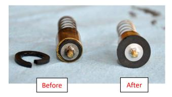
11. Examine the bypass piston; replace the rubber seal and retaining ring on the bypass piston with the new parts provided, if needed.
