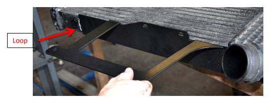
NOTE: Place the tab in the loop on the side of the CAC.
