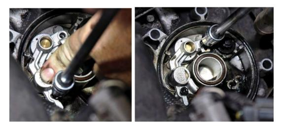
15. Install two #12 JIC 0° fittings into the Half Kit adapter.
