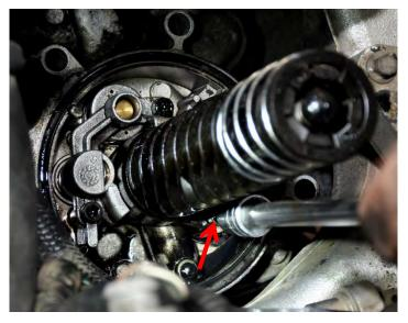
5. Remove the Torx head bolt holding down the oil filter support stand.
