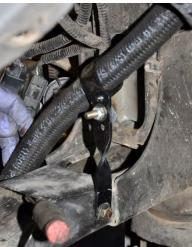
Route the 46.5" hose #2 under the radiator and over the frame rail to the #12 JIC 90° fitting on the oil filter adapter, as shown below.
