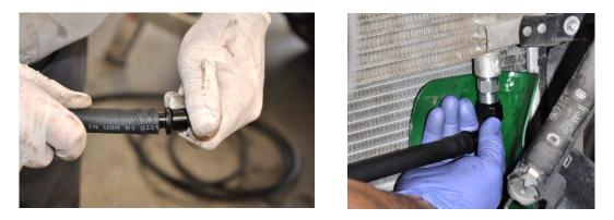
2. Route the hose along the bottom of the transmission cooler and behind the hose connected to the opposite side of the cooler. Secure the hose with the cable tie provided.
