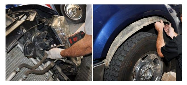
4. Remove the transmission cooler line.
