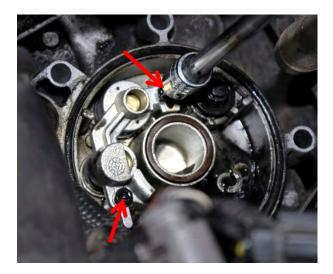
7. Remove the 2 Torx head bolts holding the stock bypass/anti-drain back assembly in place.
