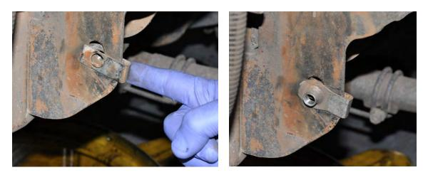
5. Mount the oil filter bracket on the truck using the stock hardware.
