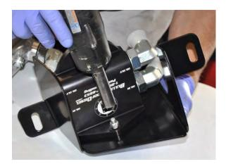
2. Attach the oil filter adapter to the oil filter bracket.
