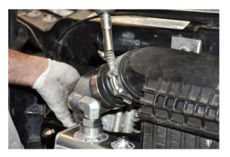
11. Reconnect the CAC pipe to the CAC. Make sure the clamp is rotated so it does not hit the hood.
