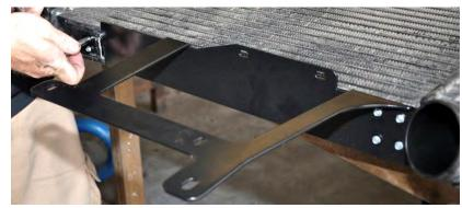
NOTE: Do not over-tighten. Stripping the screws will cause the bracket to be loose. NOTE: Only use the hardware provided! Use of longer hardware may damage the CAC.
