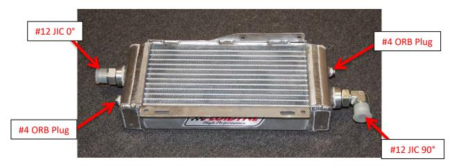
4. Place the oil cooler onto the oil cooler bracket.
