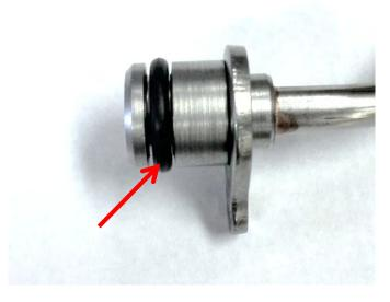
18. Reinstall the turbo oil feed line.
