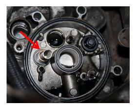
9. Once the bypass/anti-drain back assembly is removed, a spring and the bypass piston will be exposed. Remove both parts. Discard the spring.
