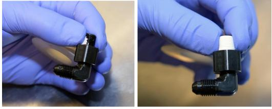
2. Install the 90° swivel fitting into the Bullet Proof Diesel oil fill cap.
