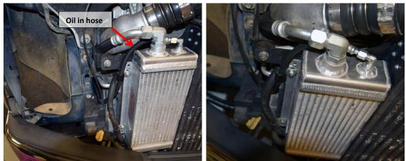
**NOTE**: Ensure the 90° fitting is not in contact with the air charge cooler inlet tube, or the main oil cooler outlet.
