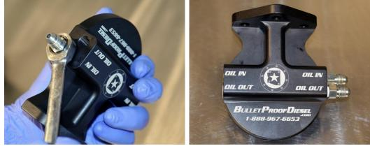
c. Using the supplied hardware, assemble the oil bypass filter adapter to the bracket.
