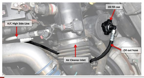
12. Securely install the "oil out" hose to the Bullet Proof Diesel oil fill cap.
