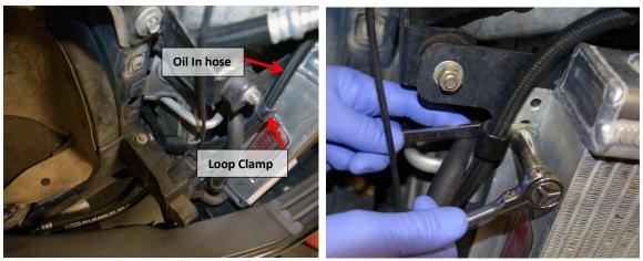
Bring the "oil in" hose to the back side of the main (larger) outlet on the half kit oil cooler. Next, connect the "oil in" hose to the ORB (O-ring boss) fitting on the 6.4L Bullet Proof Diesel half kit; the smaller bypass outlet to the right of the main outlet.
