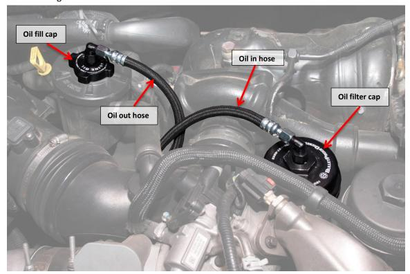
12. Securely install the "oil out" hose to the Bullet Proof Diesel oil fill cap.
