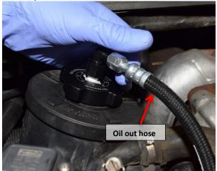
13. Securely install the "oil in" hose to the Bullet Proof Diesel oil filter cap.
