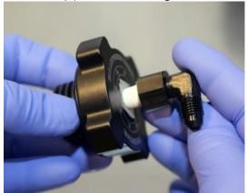
3. Install one (1) 90° swivel fitting into the Bullet Proof Diesel oil filter cap.
