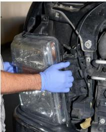
NOTE: Please remove ALL four (4) screws before attempting to remove headlight assembly. Failure to do so can result in damage to the headlight and assembly.
