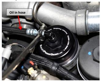
14. Ensure oil bypass bracket assembly is properly tightened down, then start the engine and check for leaks.
