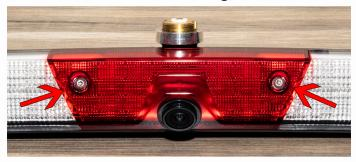
Remove the screws and seperate the adapter from the lens.
