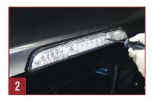
**Step. 3** Disconnect the light housing at the pigtail connector - not at the light. You may have to press down on a set of retaining clips to access the connector. Set aside the housing in a safe place for later.
