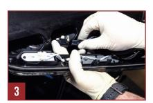
**Step. 4** Align the adapter and attach it to the cab using the four (4) factory mounting holes and the four (4) provided phillips pan screws.
