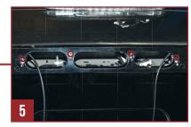
**Step. 5** Keep the adapter secured and using the four (4) top center holes as a guide, drill through the body using a 3/16" bit.
