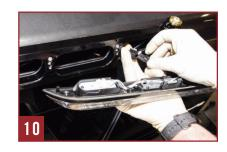
**Step. 11** Re-install the light housing using the two (2) longer cap head screws provided in the middle holes and the two (2) shorter cap scews in the outter holes. Once properly aligned, snug all the screws.
