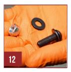
**Step. 12** Now, install the other two torx screws with washers through the two lower holes in the plastic spare tire holder and install the provided nuts and washers to the back to secure the mount.
