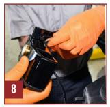
**Step. 8** Slide the third brake light wiring into the driver's side antenna mount leg. Slide the leg into the antenna mount. Secure the leg by using two of the provided M5 Cap Screws.
