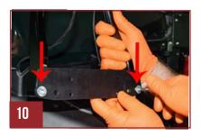
**Step. 10** Using the steel bracket provided, install the provided Flat Head Screws into the bottom holes of the antenna mount legs as shown.
