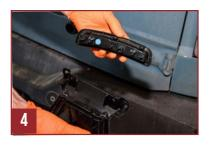
**Step. 5** Route the brake light wiring through the drivers side of the antenna mount.
