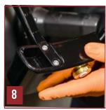
**Step. 9** Slide the antenna cable into the passenger side antenna mount leg and slide the leg into the antenna mount. Secure the leg by using the two remaining M5 Cap Screws.
