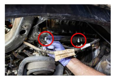
15. Now install and tighten the two nuts onto the rubber isolator studs.
