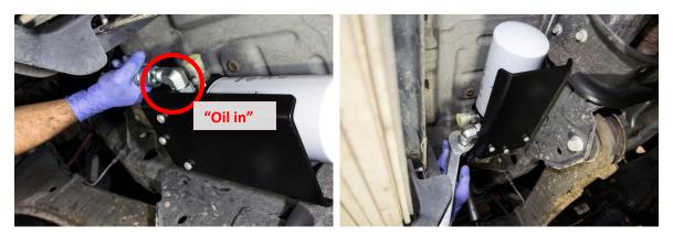
7. Next, connect the 90°x0°, 88" hose by guiding the straight end of the hose up into the engine compartment through the wheel well as shown. Guide the 90° fitting alongside the other oil line to the oil filter housing. Tighten the 90 degree end of the hose to the straight fitting, or the "Oil Out" on the Oil Filter Housing.
