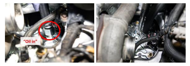
**NOTE:** With all hoses and fittings installed and tightened, check clearances with anything they might rub on and adjust accordingly, you may need to loosen and retighten hoses to properly readjust.
