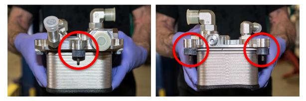
Install the coolant hoses onto oil cooler assembly.
