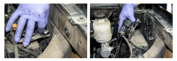
6. Unclip all four retainers to release the fuse box from its bracket.
