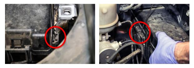
7. Accessing from the inner fender well, unclip wiring harness from the fuse box bracket.
