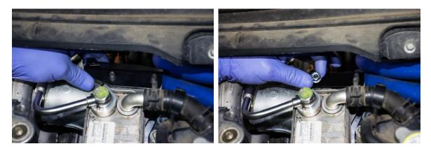
3. Install the rubber dipped clamps on to the coolant hoses, then slide the bolt through the rubber dipped clamps and tighten to the bracket.
