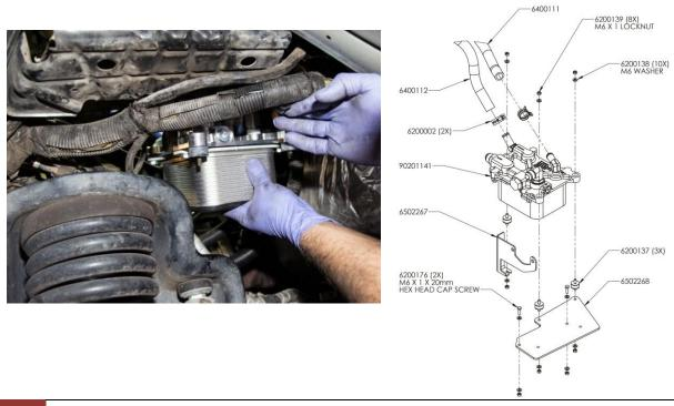
12. Using the supplied hardware, drop the 2 (two) bolts through the existing holes in the fuse box bracket.
