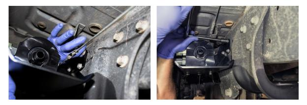
5. Install the provided filter onto the oil filter adapter.
