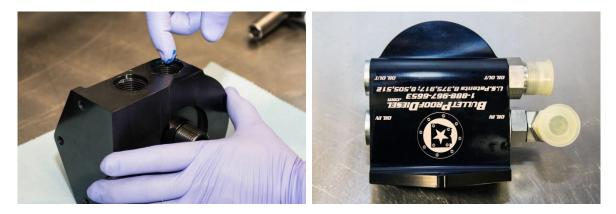
2. Using the supplied hardware install the oil filter adapter onto the oil filter mounting bracket. Be sure the longer of the 3 (three) bolts is installed into the middle hole on the oil filter adapter, using the washer and nut on this bolt only.
