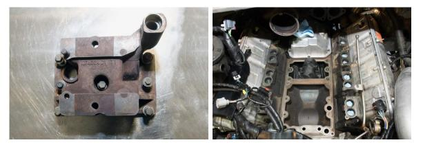
3. Install the provided seals into the bottom of the oil transfer plate; be sure to fully seat the seals into the transfer plate.
