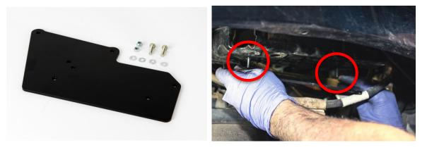
14. Once the bracket is in place, install the two retaining nuts on the bracket.
