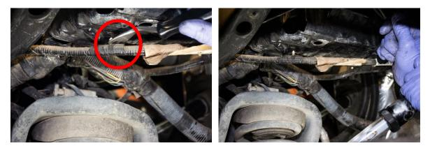
8. Use the three supplied nylock nuts and washers to attach the three rubber isolators to the oil cooler assembly as shown.
