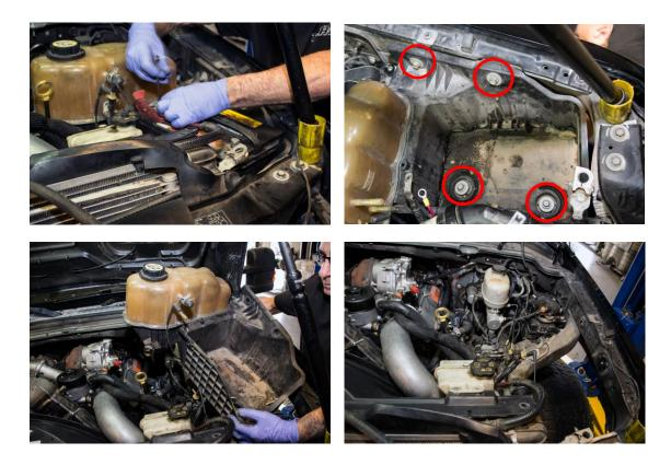
3. Remove the 2 (two) retaining nuts from the brake master cylinder.
