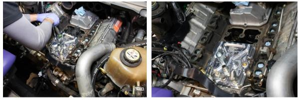
6. Using the provided seal, remove and replace turbo pedestal mounting seal. Reinstall turbo pedestal.
