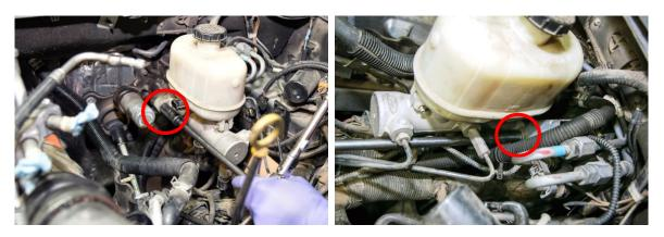
4. Using the supplied bracket, install over the brake master cylinder studs and replace the two retaining nuts.
