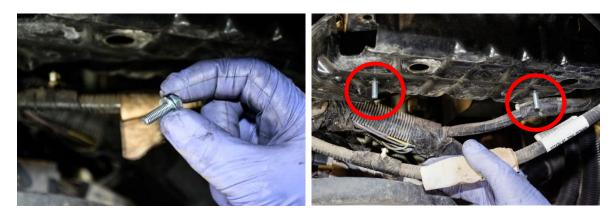
13. Slide the oil cooler bracket into place, making sure to locate the rubber isolator with the appropriate holes in the oil cooler bracket.
