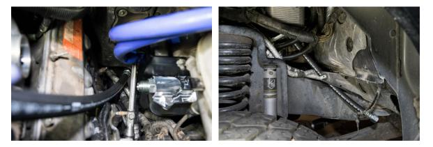
5. Connect the 90° fitting on the top side to the "Oil Out" fitting on the OEM Engine Oil Cooler Plate.
