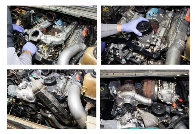
Note: Leave the u shaped portion of the turbos on the driver's side of the engine off until the oil cooler/oil cooler plate is installed and hoses are hooked up, this will come in the next section of the manual.
