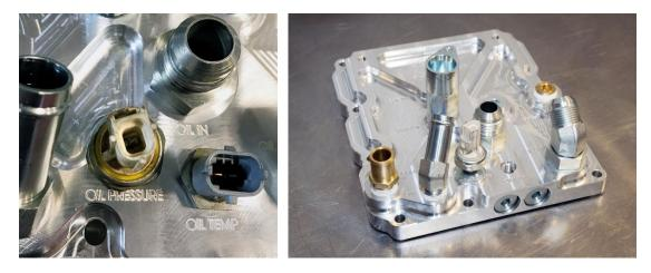
5. Using the OE oil cooler housing hardware, install the transfer plate onto engine.
