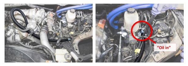
4. Install the 90°x0° 38.5" hose by guiding the straight end of the hose down towards the oil filter housing, guide the hose to the left of the steering rod as shown.
