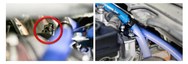
Install the coolant hoses onto the transfer block.
