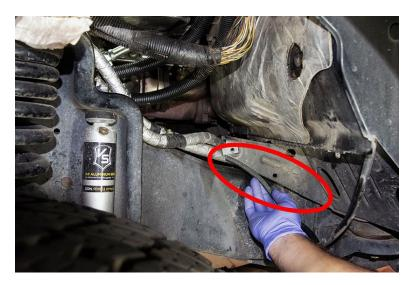
2. Install the 45°x0°, 45.5" hose by connecting the 45 degree fitting to the "Oil Out" fitting on the engine block as shown.
