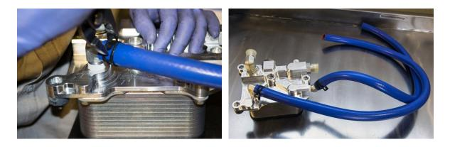
10. With coolant hoses installed, slide the oil cooler / hose assembly through the void on the inner fender on the driver's side. Guide coolant hoses over turbo while sliding oil cooler into place.
