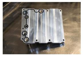
4. Remove your existing oil temperature sensor and oil pressure sender from the OE oil cooler cover and install those into their respective holes in the oil transfer block.
