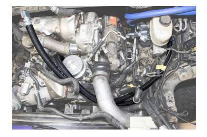
10. Attach the straight end of the hose to the straight "Oil In" Fitting on the Engine Oil Block. Use the supplied 32mm crow's foot wrench for this install.
