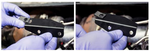
2. Index the bracket on to the fuel cooler mounting studs. Install the two retaining nuts.
