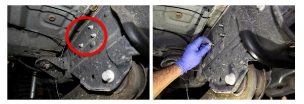
4. Slide the oil filter adapter bracket onto the three studs and reinstall the three nuts.
