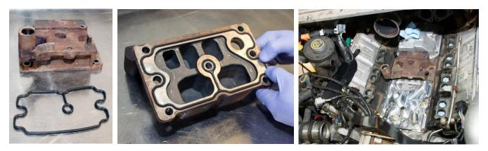
7. Once the oil transfer block and turbo pedestal have been reinstalled, reinstall the intake manifold and the turbo chargers as per OE procedures.
