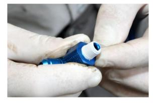
2. Install the swivel fitting into Bullet Proof Diesel Oil Filter Cap and Bullet Proof Diesel Oil Fill Cap.
