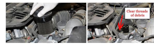
Remove the OEM oil fill cap.
