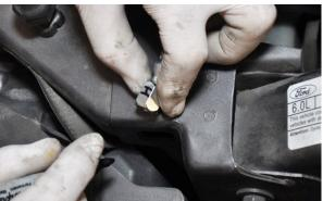
5. Push both hoses through the rubber barrier and down towards the bypass filter.
