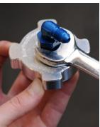
3. Install the O-ring and Oil Filter into the Bullet Proof Diesel Oil Filter Cap.
