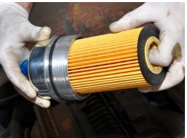
4. Install the Bullet Proof Diesel Oil Filter Cap.
