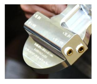
3. Install both 1/8" brass pipe plugs on the other side of Oil Filter Adapter.
