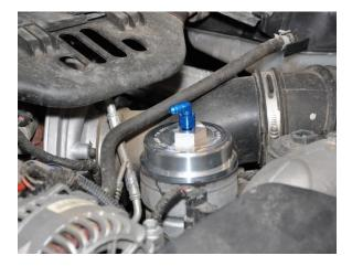
Install the Bullet Proof Diesel Oil Fill Cap on the standpipe.
