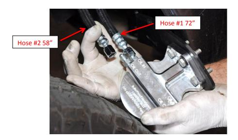
4. Place the assembly behind the bumper mount. Make sure to place the bracket between the backside of the bumper mounting bracket and stock nut retainer as shown below:
