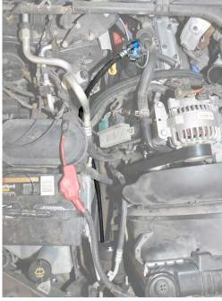
2. Route the oil hose as shown under the intercooler pipe down to rubber barrier.
