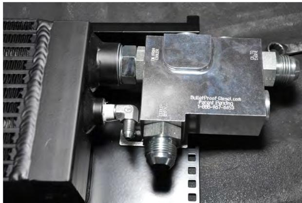
4. Before re-installing the oil cooler attach the 22 inch hose to the 90° fitting.
