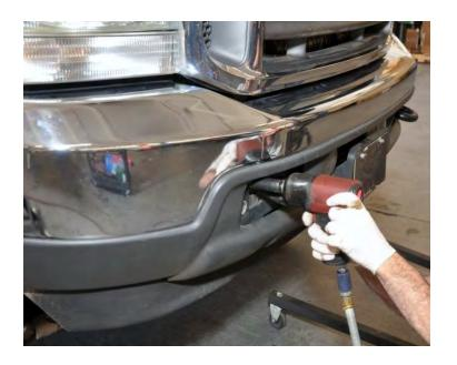
2. Remove the stock bumper support bracket. This will be replaced with a new rock shield.
