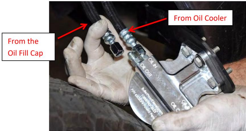
4. Place the assembled bracket behind the bumper supports. Make sure to place the bracket between the backside of the bumper mounting bracket and stock nut retainer as shown below:
