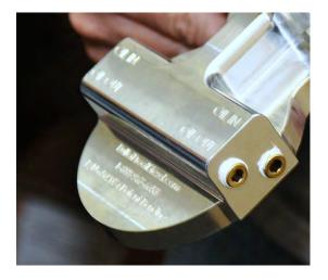
3. Install both 1/8" brass pipe plugs on the other side of Oil Filter Adaptor.
