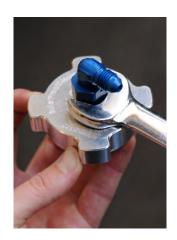
Install the swivel fitting into the Bullet Proof Diesel Oil Fill Cap. 3. Install the Bullet Proof Diesel Oil Fill Cap on the standpipe.
