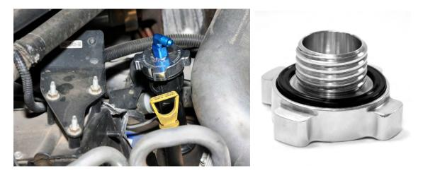
NOTE: Make sure the O-ring on the bottom of the Oil Fill Cap is in place before installation.
