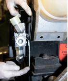
3. Replace the bottom bolt on the passenger side with provided cap head bolt.
