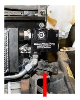
4. Make sure to get the oil cooler positioned all the way to the driver's side of the vehicle.
