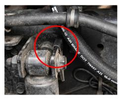
Install the edge protector on the upper shock mount to protect the hose from chafing.
