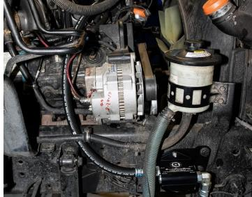
To avoid hose chafing install the screw thread protector on the valve cover bolt.
