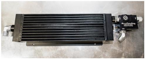
7. The O-ring boss style fittings that are used can be set at different depths. Make sure to adjust BOTH the 90° and the thermostat so that the hardline connection is lined up properly, once they are properly aligned, tighten the jam nut on both the 90° fitting and the thermostat. Once the Jam nuts are tightened, set the hard line aside you are ready to mount the cooler to the bracket.
