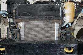
2. Install oil cooler to core support, install the spacers between the oil cooler bracket and core support PRIOR to tightening the bolts down.
