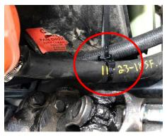
Once the hose routing is complete be sure to install the hose strap to keep the degas bottle hose and oil line from rubbing on each other.
