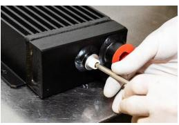
6. Install the 90° fitting onto the other side of the air cooler hand tight
