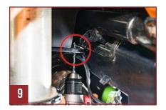
**Step. 9** Locate the plastic tray towards the top right of the oil cooler above the exhaust tube. Use your drill and 1/4" drill bit to carefully drill a hole in the corner of the tray, leave enough room so it will be a secure fit for the hose guide.
