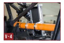
**Step. V-4** Install the oil cooler to the back bar on the passenger side as shown - leave the brackets loose for now.
