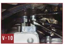
**Step. V-9** Guide the short hose through the front hose clamp then to the oil cooler.
