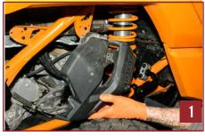
**Step. 3** Remove the (2) bolts securing the second plastic cover guard (under the hoses), remove the cover. Set aside.
