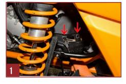
**Step. 2** Carefully clip the zip ties off of the hoses shown, there were a total of 12 on ours. Once the zip ties are removed wiggle the hoses loose.
