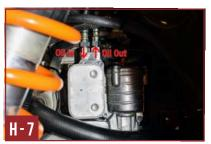
Step. H-8 Loosely install the long hose following the short hose running it through the back side of the hose retaining bracket. Connect to "Oil In"  $(\downarrow)$  on the oil cooler. Pull all the lines snug making sure they are clear from obstructions. Tighten all hose fittings and the hose clamp.
