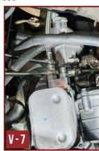
**Step. V-6** Route the hose through the front position of the hose clamp fitting.
