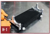
**Step. H-2** Find the (2) Port Reducers. Install the adapters onto the air-to-oil cooler. \*NO TAPE IS NECESSARY\* Tighten the fittings.
