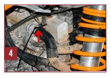
**Step. 4** You can use a large zip-tie or bungee to secure the loose hoses up out of the way so you can access the oil cooler.
