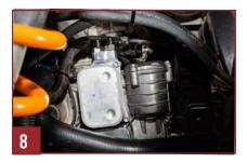
**Step. 6** Find the Oil Cooler Sandwich Plate and the (2) two -6 ORB Straight Threaded Connectors. Install the connectors to the Sandwich Plate with the o-ring side toward the plate. Tighten.
