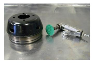
During the install of the Fan Clutch Adapter, please check your water pump pulley for a "glaze" that may have formed over time.
