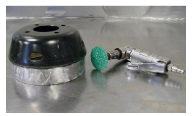
Using a heavy grit sandpaper, emery cloth, or sanding disc, use moderate force to scuff up the pulley in the area where the belt rides.
