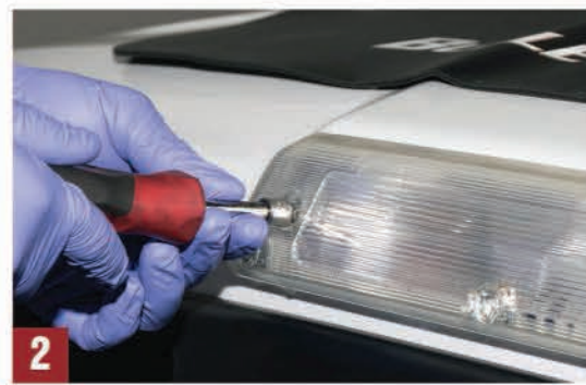
Fig. 2-3 Using a 9/32" (7mm) nut driver remove the two (2) screws holding the housing in place and pull away from the cab. Fig. 4-6 Disconnect the harness from the housing by rotating the bulbs counter-clockwise, then pull straight out to remove from the housing. Disconnect the power harness by pressing down on the retaining clip, then slide away from the housing.
