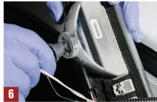
Fig. 2-3 Using a 9/32" (7mm) nut driver remove the two (2) screws holding the housing in place and pull away from the cab. Fig. 4-6 Disconnect the harness from the housing by rotating the bulbs counter-clockwise, then pull straight out to remove from the housing. Disconnect the power harness by pressing down on the retaining clip, then slide away from the housing.
