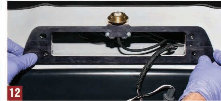
Fig. 7 Route the antenna cable into the cab following the brake light harness. From inside the cab, access the cable and route to final desired location. Fig. 8 Route the bulbs and harness through the middle of the antenna adapter. Fig. 9-12 To attach the antenna adapter, position it just below the top of the opening on the cab to allow the support tab to clear the sheet metal. With the tab through the opening, slide up to align with the factory mounting holes. Fig. 13-14 Using the factory installation screws, temporarily attach the adapter utilizing the factory mounting holes and hardware. Tighten the two (2) support tab screws to sandwich the cab between the tab and the adapter to finish adapter install. Fig. 15 With the adapter in place, secure with the provided self-tapping screws and 1/4" nut driver. NOTE: Use of power tools can make hardware installation easier, but use CAUTION since you are working near a painted surface. Fig. 16 Remove the factory installation screws.
