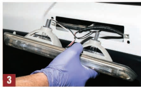
Fig. 2-3 Using a 9/32" (7mm) nut driver remove the two (2) screws holding the housing in place and pull away from the cab. Fig. 4-6 Disconnect the harness from the housing by rotating the bulbs counter-clockwise, then pull straight out to remove from the housing. Disconnect the power harness by pressing down on the retaining clip, then slide away from the housing.
