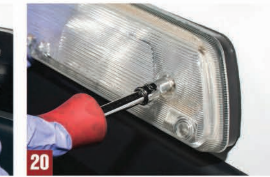
Fig. 17-18 Attach the bulbs and power connector in the reverse manner as removal. Fig. 19 Route the harness and back of the light housing to avoid interference with the antenna cable, as it is positioned back in place. Fig. 20 Re-install the light housing utilizing the factory hardware. With the 3rd Brake Light Antenna Adapter installed, attach desired compatible antenna with NMO standard threaded antenna connector and fasten the PL-259 male UHF connector to preferred 2-way radio.
