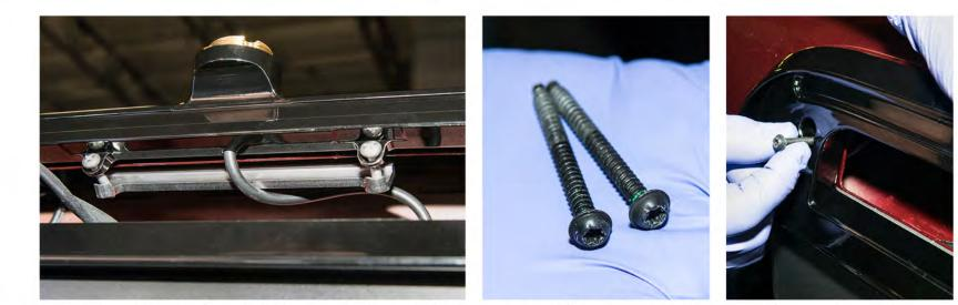
Route the cable into the cab following the brake light harness. Seat the adapter as shown. Use the two OEM T20 screws to secure the antenna adapter to the cab using the factory holes.
