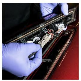
Disconnect the wiring harness and set the brake light housing aside.
