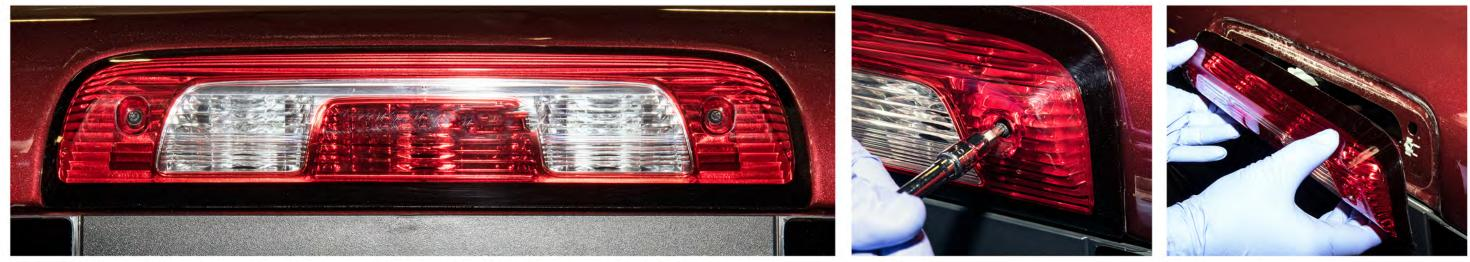
Using the T20 Torx Driver, remove the two screws holding the brake light housing in place and pull the brake light away from the cab.
