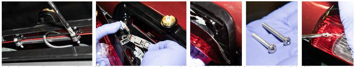
Tighten the screws on the antenna mount clamp until they are snug. Reconnect the wiring harness and guide the pin from the brake light housing into the machined holes of the antenna mount. Use the supplied screws to secure the OEM brake light housing to the antenna adapter.
