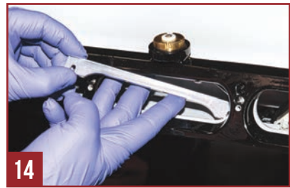
Fig. 13-15 Keep the adapter secured in place. Using the adapter's two (2) top center holes as a guide, drill through the truck body with a 3/16" bit. Next, feed the support bracket through the middle hole of the adapter. Slide the support bracket behind
