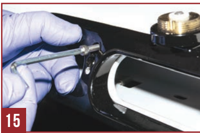
Fig. 13-15 Keep the adapter secured in place. Using the adapter's two (2) top center holes as a guide, drill through the truck body with a 3/16" bit. Next, feed the support bracket through the middle hole of the adapter. Slide the support bracket behind
