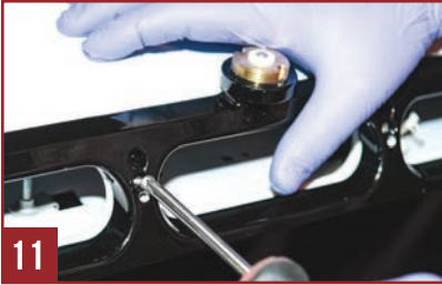
Fig. 9-12 To attach the antenna adapter, align and attach the adapter utilizing the four (4) factory mounting holes and the provided phillips pan head screws.
