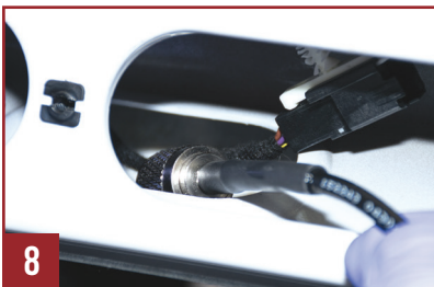
Fig. 8 Route the antenna cable into the cab - follow the brake light harness. From inside the cab, access the cable and route to final desired location.
