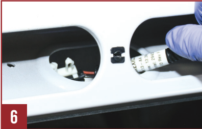
Fig. 4-7 Disconnect the light housing at the pigtail connector - not at the light. Access the connector by pushing down on the clips and pulling through the opening on the right.
