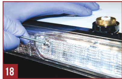
Fig. 17-19 Re-install the light housing utilizing the provided longer button head cap screws for the middle two (2) holes and the shorter button head cap screws for the outer two (2) holes. With the 3rd Brake Light Antenna Adapter installed, attach
