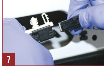
Fig. 4-7 Disconnect the light housing at the pigtail connector - not at the light. Access the connector by pushing down on the clips and pulling through the opening on the right.
