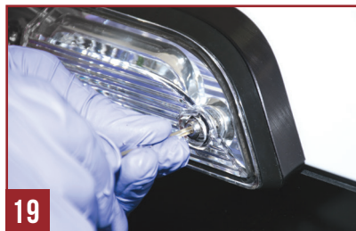
Fig. 17-19 Re-install the light housing utilizing the provided longer button head cap screws for the middle two (2) holes and the shorter button head cap screws for the outer two (2) holes. With the 3rd Brake Light Antenna Adapter installed, attach
