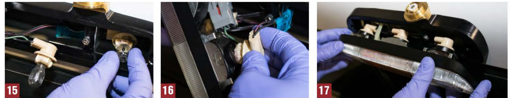
Fig. 16 Route passenger side cab light bulb behind the support bracket and back through the antenna adapter opening. Fig. 17-18 Attach the bulbs to the light housing starting with the passenger side, then middle brake light bulb and finally the driver side. NOTE: The power connectors WILL NOT be re-attached to the anchor point on the light housing. Route the harness and back of the light housing to avoid interference with the antenna cable as it is positioned back in place. Fig. 19 Re-install the light housing utilizing the provided hardware. With the 3rd Brake Light Antenna Adapter installed, attach desired compatible antenna with NMO standard threaded antenna connector and fasten the PL-259 male UHF connector to preferred 2-way radio.
