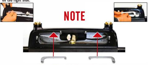
THESE TWO BRACKETS SLIDE BEHIND THE CAB FRAME - YOU WILL NEED TO SECURE THEM WITH THE SUPPLIED HEX SCREWS.
