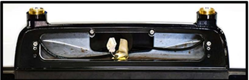
6 - Reinstall your OE Brake Light to the BulletProof Antenna Mount using the two (2) supplied Phillips screws. Be sure to reattach the brake light connector.
