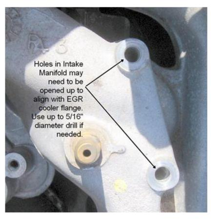
Due to the variation in the EGR cooler flanges, it may be necessary to drill out the holes in the Intake Manifold. Use up to a 5/16 inch diameter drill if needed.
