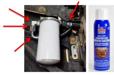
Some of our customers live in areas/climates where salt or chemicals are used for deicing the roads in the winter months. These substances can cause premature deterioration of the fittings and hoses.
