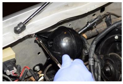
6. Tighten the provided M6 bolt onto the vacuum reservoir ball.
