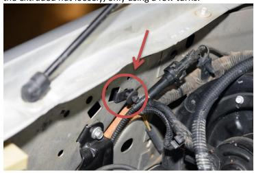
5. Slide vacuum reservoir ball onto the installed bolt and install self-tapping screw into truck body.
