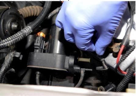
2. Disconnect the vacuum line as shown.
