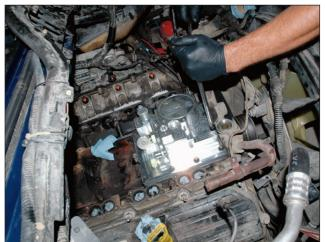
After bolting the transfer block to the top of the engine, ¾-inch high-pressure Goodyear oil lines and -12 JIC (Joint Industry Conference 37-degree flared fittings) were routed.
