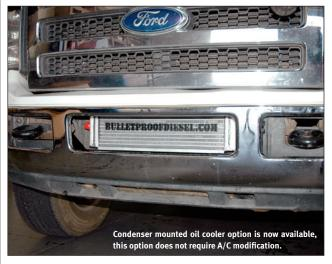
The bumper-mounted Fluidyne air-to-liquid cooler was bolted in front of the A/C condenser. If A/C performance suffers, BPD recommends removing the OE orifice tube and replacing it with a GM white orifice tube (Four Seasons Part# 38623) after reclaiming the original refrigerant. Then recharge the A/C system with an additional 6 ounces of refrigerant more than the OE specified amount. Perform a testdrive at highway speeds and add up to an additional 12 ounces of refrigerant as needed.
