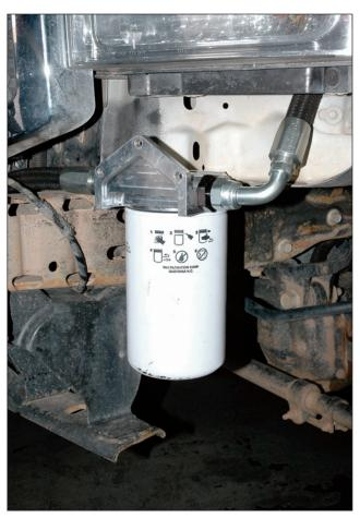
The oil lines and -12 JIC fittings were routed to a Wix 85832 spin-on filter remotely mounted with a custom bracket since the factory bumper—where BPD usually mounts the 18½-gpm filter—had been replaced with a large, tubular, steel winch bumper.
