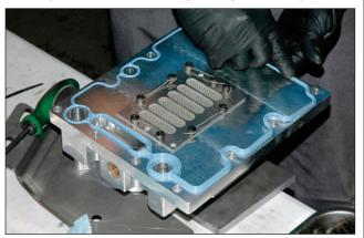
Here is the backside of the BPD billet aluminum oil transfer block (replacing the factory oil cooler and filter block) with its steel screen (replacing the factory plastic screen) bolted and safety-wired so there is no chance of anything coming loose and falling into the HPOP.
