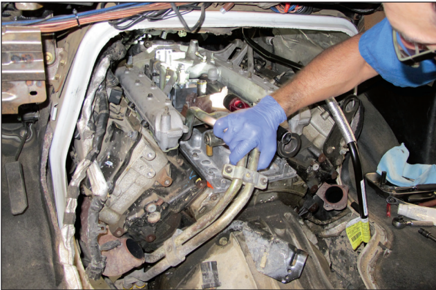
The factory remote-mount oil filter lines were then connected to the BPD oil cooler module using the factory hardware and new O-ring seals.
