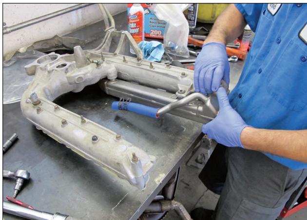
The BPD oil cooler module was then bolted into place using the factory hardware.
