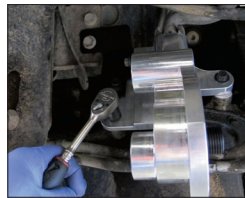
The factory remote-mount oil filter lines route the engine's oil down to the driver's side of the engine.
