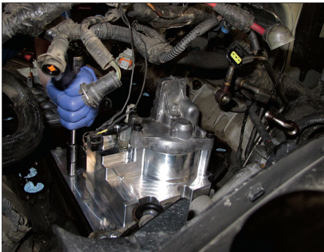
The BPD oil cooler module was then bolted into place using the factory hardware.
