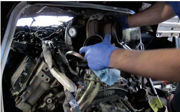
The factory wiring harness was then reconnected, and the Garrett VGT turbo was hoisted into place. It was at this point Lopez noticed the transmission dipstick tube was cracked, so he installed a replacement unit before bolting the exhaust manifold up-pipes and downpipe in place.
