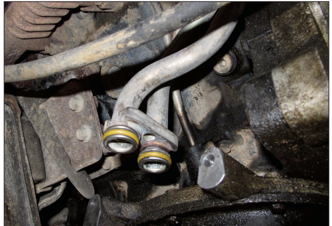
The factory remote-mount oil filter lines route the engine's oil down to the driver's side of the engine.
