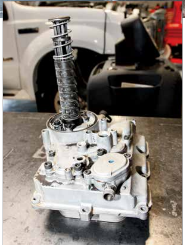
This is what we are replacing. Tucked deep in the engine's valley, underneath the intake manifold, is the oil transfer block. Note: The factory oil filter housing has been removed in this photo.
