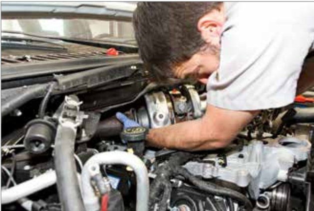
Next up was reinstalling the turbocharger, which had received a thorough cleaning while it was removed, ensuring many more years of trouble-free service.
