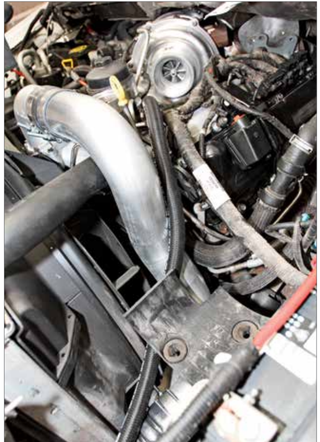
From this angle, you can clearly see the proper routing of the driver-side hose, which skirts around the intercooler pipe and under the airbox.
