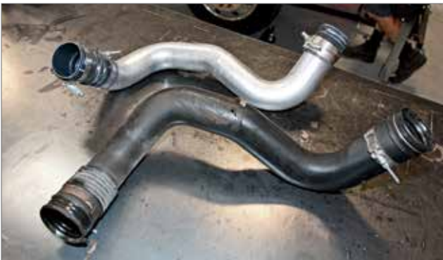
Throughout its short lifespan, the 6.0L was subjected to a multitude of design changes, one of which was the change from a metal to plastic cold-side intercooler pipe during the '05 model year. Swapping in the older-style pipe is a simple bolt-on affair, and Bullet Proof recommends it for anybody with the new plastic-style pipe. This simple change can prevent many headaches down the line.
