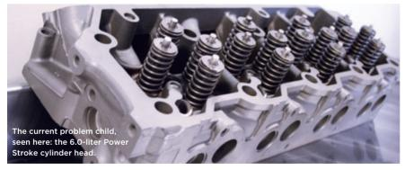
here are few experiences in life more unpleasant than opening up one's cooling system and finding something other than coolant. If you have diesel fuel in the coolant of your 6.0-liter Ford Power Stroke, there's a very good chance you've stumbled upon one of the engine's weak points: a crack in the cylinder head between the injector bore and the coolant passage. Ford's recommended repair? Replace the head.
