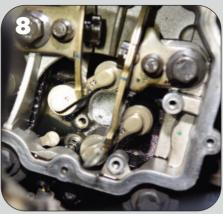
WD-40 and allow it to settle. Now comes the part that requires patience. Look for bubbles coming from the exhaust manifold side of the bore. An inspection mirror will be helpful for the rear cylinders. Cracks are most commonly found in cylinder number five (second from the rear on the passenger's side), but Bullet Proof has found cracks in all eight cylinders. Once the cracks have been found, sponge out the WD-40, again using dry shop towels. You are now ready to begin the
