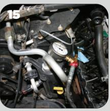
Watch the gauge for 10 to 15 minutes. The pressure should drop slowly. No pressure drop indicates that either there's no crack at that cylinder or the tool is improperly installed.
