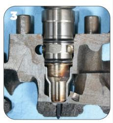
This photo shows where the damage occurs. Fuel enters from the fuel rail (the circular opening at the left), and the crack is on the right. above the injector cup. Mechanics familiar with the 7.3 may misdiagnose the problem as a broken injector cup. On the 6.0 engines, the cracks occur in the head, above the cup
