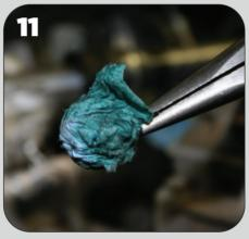
Place a wad of paper towel into the injector bore to prevent sealant from seeping into the cylinder. The repair tool is installed using the factory injector hold-down bolt. Hand-torque the tool to 24 ft.-lb., working slowly and gently to ensure the tool remains centered and does not bind.
