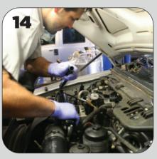
A grease gun is used to pressurize the sealant. Prime the pressure gauge and hose (included with the kit) until grease runs out of the end; air in the hose will give a false pressure reading. Attach the hose to the repair tool and pump the gun until the pressure stabilizes at 500 psi. Do not pump more than necessary, otherwise you may force grease into the crack, which will require re-doing the repair.
