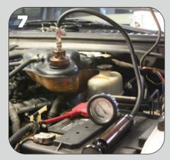
Using a coolant system pressure tester, pressurize the cooling system to 20 psi.
