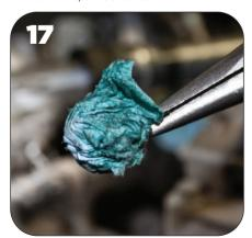
Remove the towel from the injector bore. Clean the bore using a dry shop towel, lube the O-ring and tool, and repeat the repair procedure for other cylinders with cracks.
