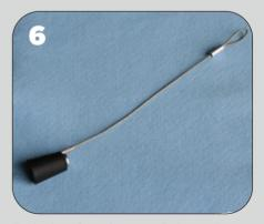
Testing is performed on one cylinder at a time. Cracks may exist in more than one cylinder, so be sure to test all eight. Install the four rubber stoppers, which are included with the kit, into the injector bores on one side of the engine. Reinstall all parts removed to drain the coolant (block plugs, petcocks, etc.) so that the cooling system can be pressurized.
