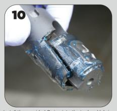
Install the provided O-ring into the tool and lubricate it with transmission assembly lube or grease. Lubricate the entire bottom part of the tool as well as the slide sections between the moving parts of the tool. Without proper lubrication, the tool may bind when you try to remove it.
