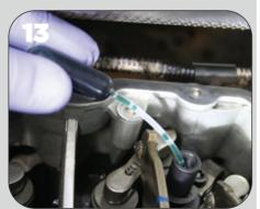
Fill the tool with the sealant. Each pipette contains enough sealant for one cylinder
