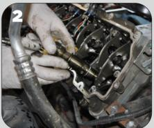
Repair starts by draining the radiator and re moving the block plugs to drain coolant from the engine. The cooling system must be completely drained. Next, remove all eight fuel injectors following the procedure in the Ford service manual
