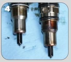
If the crack has extended below the lower injector O-ring, the injectors themselves may give some clue as to the location of the leak. The injector on the left has a small rust stain near the tip, which indicates contact with coolant pooled in the bore. The residue on the injector at right is from coolant-contaminated fuel, and may indicate a leak upstream (i.e., a lower cylinder number). Clean injectors do not indicate lack of a leak; you still need to pressure-test.
