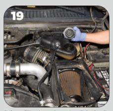
Before refilling the cooling system, Bullet Proof Diesel recommends changing all of the cooling system O-rings and hoses, which may have been contaminated by diesel fuel. (A list of recommended replacement parts is provided with the instructions.) If the degas bottle cap binds when you screw it on, the bottle or the cap may be swollen and will need to be replaced. Flush and refill the cooling system, reinstall the injectors, and the repair is finished!
