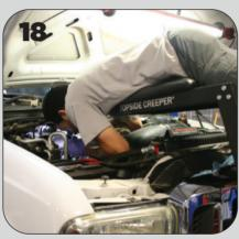
The sealant must cure for 24 hours (longer in cold temperatures). Do not turn the key to the "on" position as this could pressurize the fuel system. After the sealant has cured, re-test the repaired cylinders using the rubber stoppers, WD-40, and coolant pressure tester. If any of the cylinders show signs of leaks, repeat the repair procedure.
