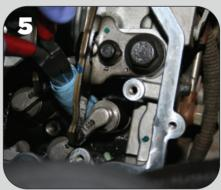
Clean the cylinder heads using a dry shop towel. Vertical marks (perpendicular to the bore) on the exhaust manifold side of the bore are indicators of a crack; machining marks for the bores run parallel to the plane of the cylinder head.
