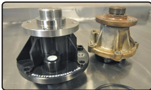
12, 13 Bullet Proof water pump next to the factory pump. The Bulletproof pump is 100-percent billet machined from high-grade aluminum and stainless steel for strength, longevity and to ensure a perfect fit with exact tolerances for problem-free performance. The aluminum impeller is much stronger than the factory plastic impeller and resists spinning on the pump shaft like the factory one can under heavy loads. The factory impeller also flexes under load, which causes cavitation that beats up on the front cover eventually leading to failure. This is virtually impossible with the Bullet Proof aluminum impeller.
