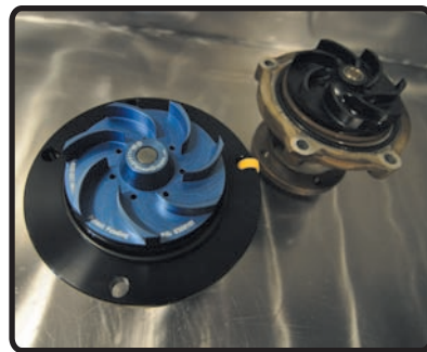
12, 13 Bullet Proof water pump next to the factory pump. The Bulletproof pump is 100-percent billet machined from high-grade aluminum and stainless steel for strength, longevity and to ensure a perfect fit with exact tolerances for problem-free performance. The aluminum impeller is much stronger than the factory plastic impeller and resists spinning on the pump shaft like the factory one can under heavy loads. The factory impeller also flexes under load, which causes cavitation that beats up on the front cover eventually leading to failure. This is virtually impossible with the Bullet Proof aluminum impeller.
