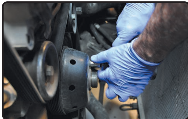
10 The water pump pulley must be removed in order to remove the factory water pump. To stop the pump from spinning, while removing the bolts securing the pulley to the pump, Del kept the accessory drive belt installed while he removed all but one bolt. The last bolt was simply loosened to then be removed later—after the belt had been removed.
