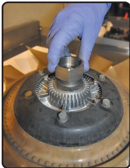
7 6.0L clutch on the right and 7.3L clutch on the left. In between the two is BulletProof's adaptor, which allows the 6.0L water pump to bolt up to the 7.3L fan as the two use a different thread size and pitch.
