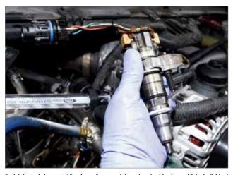
Each injector is inspected for signs of wear and then placed aside along with its individual holder. A clean working surface is vital to preventing contamination of the fuel injectors.
