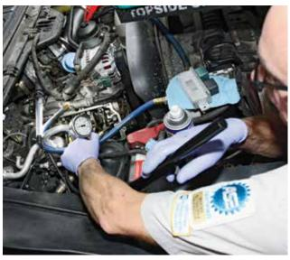
After the pressurized, solution-filled pipette sits for 10 to 15 minutes, pressure will drop as a result of the sealant making its way into the crack. Once all the cracks are repaired, the truck should be left with the injector bores open for 24 hours to allow the solution to fully cure. If everything checks out after 24 hours, the fuel system is ready to be reassembled and the truck is sent on its way.
