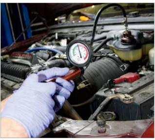
Once the bubbles in the WD-40 subside, the coolant system is drained and then pressurized to 15 psi using a hand pump and the truck's degas bottle. Finding the offending cylinder is as simple as seeing which injector bores are bubbling from the pressurized cooling system.
