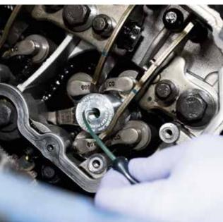
This is what makes the magic happen. A pipette is filled with the proprietary solution, which is then inserted into the top of the tool. Once full, a zerk fitting is added to seal the hole and facilitates using a grease gun to apply 500 psi of pressure to force sealant into the cracks.
