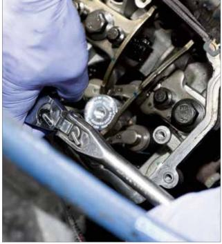
Using the proper injector retainer for the cylinder that showed symptoms, Delwin inserts the tool and torques the retainer to the proper specifications. Overtightening the retainer may cause the tool to get stuck in the bore, which won't damage the cylinder head but will render the tool unusable.
