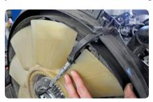
The Ford's radiator fan uses an electrically controlled clutch. The wires to this clutch always seem to get caught by the fan, and obviously, get ripped apart. Further proving
