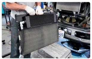
The new air-to-oil cooler mounts to the AC condenser with supplied bracket and hardware. Heavy-duty hydraulic lines connect the manifold in the engine's valley to the filter and new cooler. This air-to-oil cooler will keep the engine oil much cooler than the factory one. This means less deposit build up and better lubrication for the entire engine.
