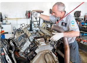
With the cab off, Bulletproof Diesel's Del Wamsley removed the turbo, intake manifold, EGR cooler, wiring, and more to gain access to the valley.
