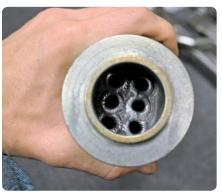
Here the new reworked **Bulletproof EGR** cooler, it's a much stronger unit consisting of six stainless steel tubes that allow less restriction in the exhaust and better coolant flow. The end result is cooler exhaust temperatures,
