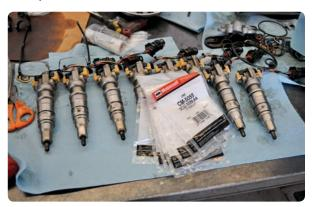
These injectors were in good shape, new gaskets and seals were installed, and they were re-installed in the heads.
