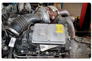
Last big problem: The fuel injection control module (FICM). It's the brain of the engine and lives its life in a very harsh environment. Mounted to the driver's side, valve cover vibration and high heat levels beat up on the FICM. A failed FICM will cause slow starts, poor cool-weather performance, poor performance, poor fuel economy and possibly a no-start situation.
