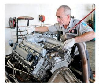
New EGR cooler and factory intake being installed.
