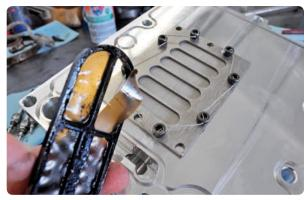
This screen is located below the oil cooler. It is there to stop contaminants from entering the injection system, potentially causing a no-start condition. They fail all the time like this one has. Bulletproof's new manifold uses a much more robust screen, which you can see in the background.
