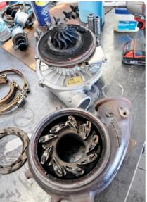
This VGT turbo uses a series of vanes to change the velocity at which the incoming exhaust air hits the exhaust turbine/wheel. To keep it simple, the end result is a turbo with almost zero spool up time that can give the engine a healthy and correct amount boost at any rpm. The problem occurs when the vanes become clogged with soot and freeze up.
