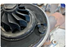
This pin/ lever controls the direction of the turbo's vanes.
