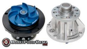
27 Another common failure is the Powerstroke's water pump. The factory pump has a plastic impeller that commonly cracks around the hub. The new Bulletproof pump uses a much stronger billet aluminum impeller, which helps prevent failures that could lead to overheating problems.
