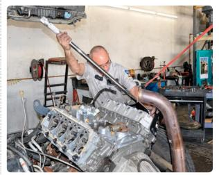
The final torque of the studs, done with ARP's Ultra-Torque on the threads, should be 210 ft.-lbs. Factory head bolts take a much less 85 ft.-lbs. of torque (plus another three-quarter turn of the wrench).
