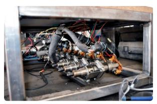
Ken Neal built this test bench where each FICM is plugged in to ensure there are zero problems before it goes out to the final user. The tester has all eight injectors set up to fool the FICM into thinking it's plugged into a running 6.0 liter.
