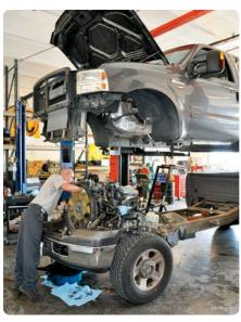
Accessing the motor for a repair like this one requires removing the cab. It's really not as bad as it looks, and only takes a couple hours to complete.
