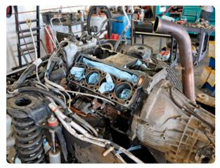
The valve seats in the heads tend to crack. So Del removed the heads and sent them out to be checked for straightness and to have the seats swapped out for hardened ones. Del then began to clean every nook and cranny of the disassembled engine until it was surgically clean.
