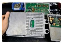
When FICMs fail, it's rarely the brain, but usually its power supply (on the right of the photo). Testing the FICM is easy. Simply measure the voltage output at the top pin (here it would be the
