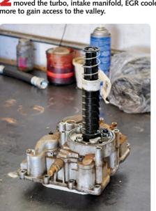
This manifold houses the factory oil cooler, a few sensors, and the factory oil filter. The black tube is what the factory drop-in filter surrounds and attaches to. Atop the tube is a bypass valve that is famous for breaking. When it does, oil completely bypasses the filter and sends contaminants straight to the high-pressure oil pump
