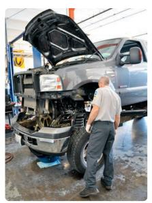
The factory power-steering cooler must be moved on this 2006 Superduty to allow room for the new oil cooler. It's a quick job as earlier Superdutys had their power-steering cooler mounted low, so the bolt holes are already there.
