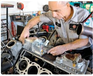
Here Del installs the new Bulletproof Diesel Transfer Block. The transfer block diverts engine oil down a hydraulic line to a new air-to-oil cooler and through a traditional spin-on filter, eliminating the problematic factory filter and cooler.
