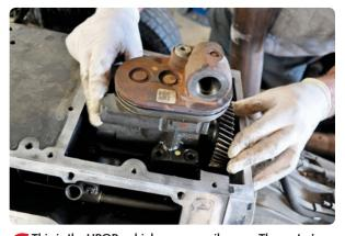
This is the HPOP or high-pressure oil pump. The motor's HEUI (hydraulically actuated electronically controlled unit injection) injectors use oil pressurized by this pump to inject fuel into the cylinders. Good, clean, and cool oil is extremely important to this power plant due to this HEUI system. Bulletproof removes and inspects the HPOP, if no problems are found, they replace all seals and reinstall it.
