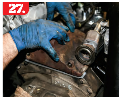
27. With the new seals in place, the pump cover is reinstalled and torqued to spec.
