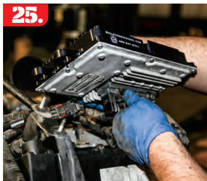
25. The now-bulletproof FICM was bolted into place above the left valve cover.
