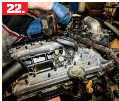
22. Using all the new seals, the intake manifold assembly was now bolted into place.
