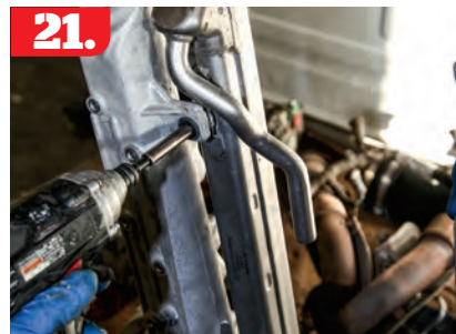
21. The previously removed intake manifold was cleaned and surfaced until it looked brand new. Then, the Bullet Proof Diesel EGR Cooler was bolted up, followed by the polished up throttle body.
