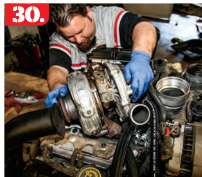
30. With the turbocharger looking better than new we buttoned it back up and reinstalled it on the turbo pedestal. At this point, the cab is dropped back down and all of the electrical is reconnected. We're in the home stretch now.
