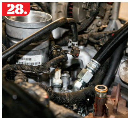
28. From here we can begin to route the oil cooler lines over toward the passenger fender where the cooler will be located.
