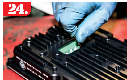
24. The stock FICM was split in half, and OE bottom half was attached to the Bullet Proof Diesel billet top section. These heavy-duty FICMs can be bumped up from 48 volts to 53 or 58 volts, but shown here, we are adjusting them to the stock output.
