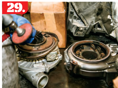
29. The factory turbo had been replaced with a rebuilt unit about a year ago, but on inspection, we decided to do some polishing before we reinstalled it.
