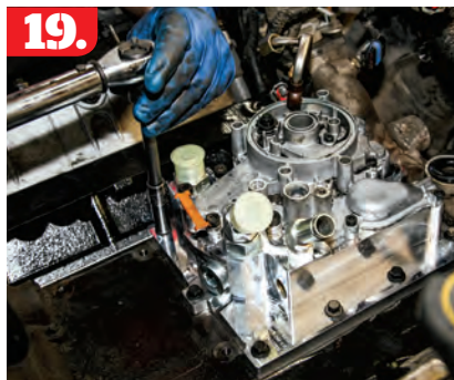
19. With no oil cooler down below, the new assembly was bolted back in place in the engine valley.
