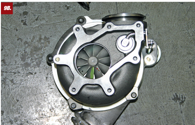
9A & B. The exhaust housing connected to the up pipes is re-used on the new turbo. You can also see that the turbine wheel blades are more aggressive than the stock turbo. The wastegate is a tad larger than stock, too.
