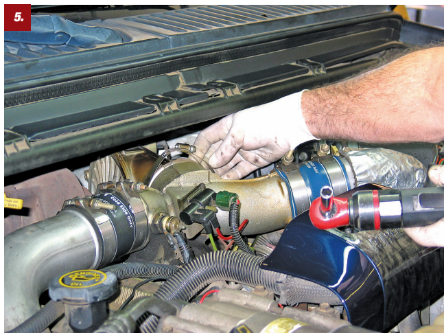
5. The install is a basic 7.3L turbo R&R. You start by removing the boost tubes from the intake manifold and all the clamps. On this truck, the Airaid intake was also unbolted for more room to get at the boost tubes.
