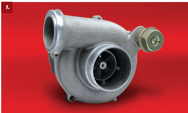
1. The GTP38R is designed as a direct replacement that utilizes the stock pedestal, oil drain back channel and oil feed. It pumps out 33 percent more flow than stock and is rated up to 40 psi.
