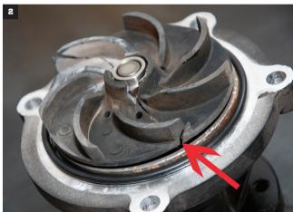
This closeup shot shows a more detailed look at the damage. The broken impeller obviously causes overheating issues, since the hub now spins
