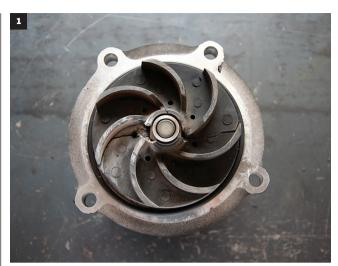
The stock water pump on the 6.0L Power Stroke features a composite (plastic) impeller that's been know to crack and fail. The damage is obvious on this impeller. Also note the score marks on the impeller fins where it hit the back of the housing.
