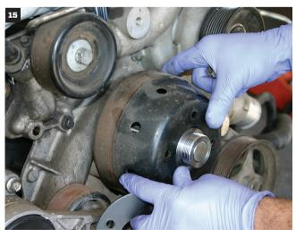
Last up, install the drive pulley and put the rest of the cooling system, (i.e., the fan and fan shroud) back on the truck. Refill with coolant—and you're done.
