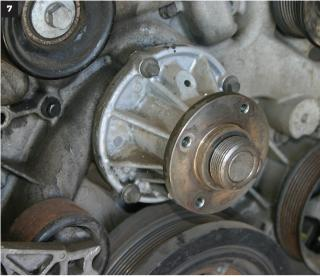
This is what sits behind the pulley: a simple, four-bolt water pump.
