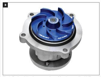
The Bullet Proof Diesel answer to the problem is an anodized hillet aluminum impeller installed on a brand-new stock water pump. According to Bullet Proof, the added rigidity of the aluminum reduces pump cavitation and damage to the water pump housing.
