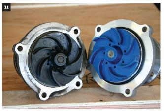
Here's a side-by-side comparison of the stock pump (left) and the new billet pump (right). Notice the difference in the overall impeller shape, which improves efficiency.
