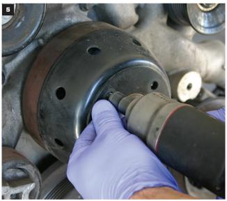
5 & 6 The outer pulley that drives the pump comes off first by removing four bolts.
