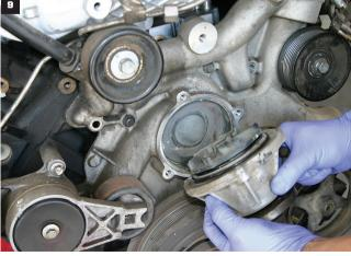
Once unbolted, the pump just pops out. And since there's an O-ring that seals the pump to the housing, you don't have old gaskets to scrape off.
