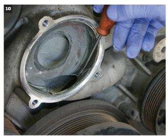
You can see where the stock pump impeller has cut a groove into the water pump housing from flex.  $\,$
