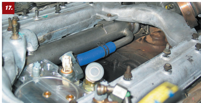
17. Once the intake manifold is bolted in place, the EGR cooler line can be attached to the oil-cooler manifold. The round-capped fittings you see on the oil manifold are fittings that connect to the remote cooler lines.
