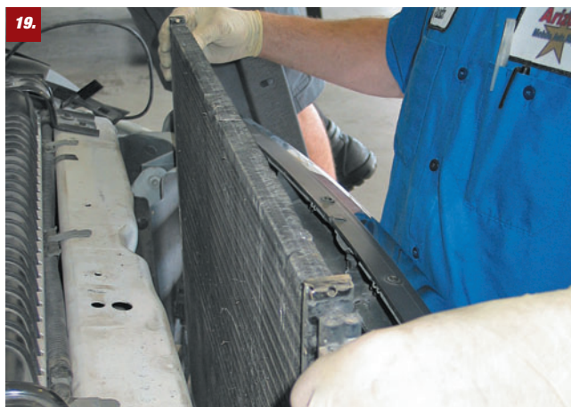
19. The A/C system is evacuated so the condenser can be removed.
