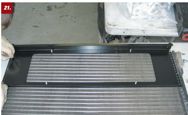
21. The kit includes this oil-cooler bracket that is mounted to the A/C condenser.
