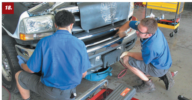
18. Installation of the Bullet Proof Diesel remote oil-cooler kit starts with removal of the stock bumper.
