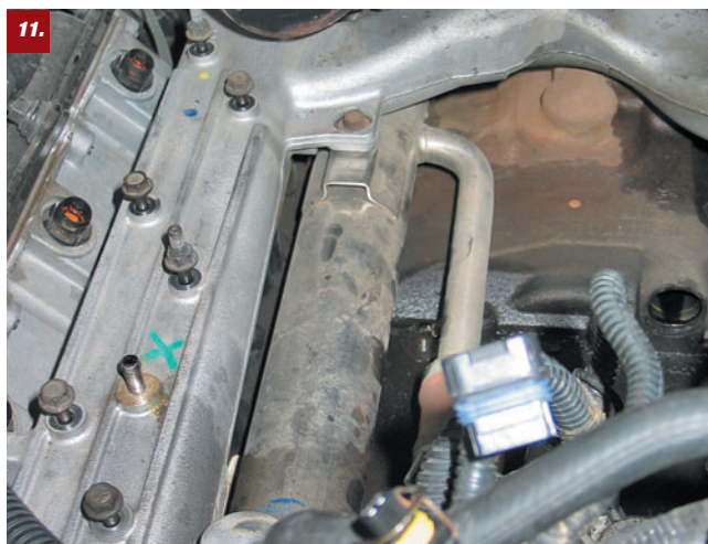
11. This shot shows the location of the stock EGR cooler, which is bolted to the bottom of the intake manifold. The manifold has to come out to do the R&R on the EGR cooler.
