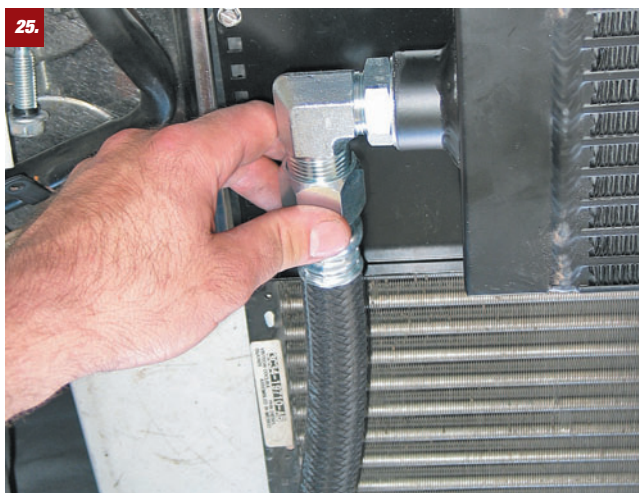
25. Braided lines deliver oil to and from the cooler.
