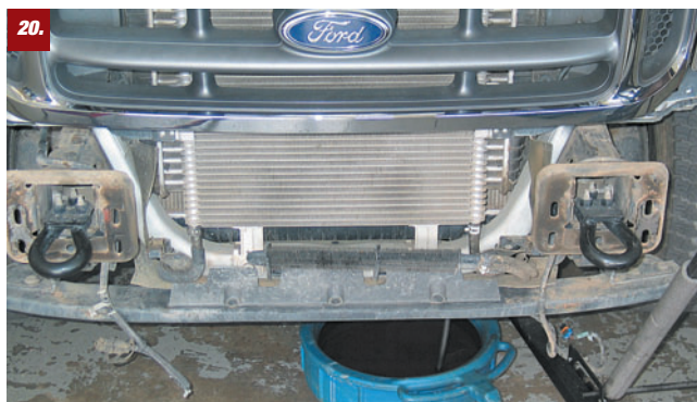
20. The factory transmission cooler will be lowered to this position via new mounting brackets to make room for the remote oil cooler that is mounted at the top of the A/C condenser.
