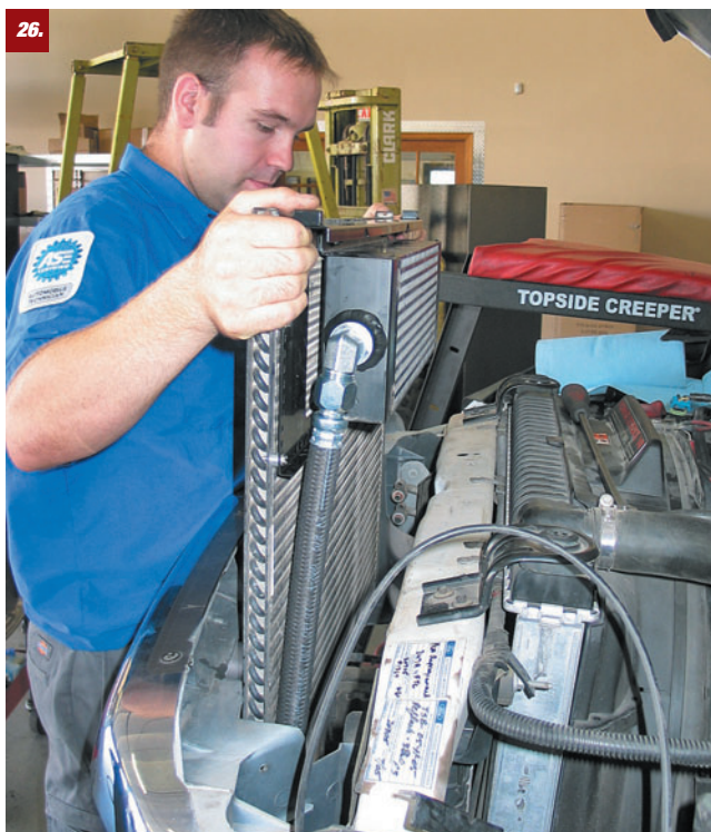
26. With the cooler and oil lines attached, it can be carefully relocated inside the truck.
