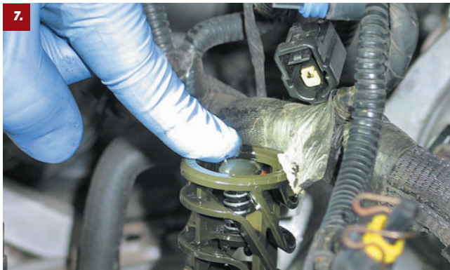
7. According to Bullet Proof Diesel, another weak point on 6.0L Power Strokes is this plastic check ball that controls the oil bypass inside the filter.
