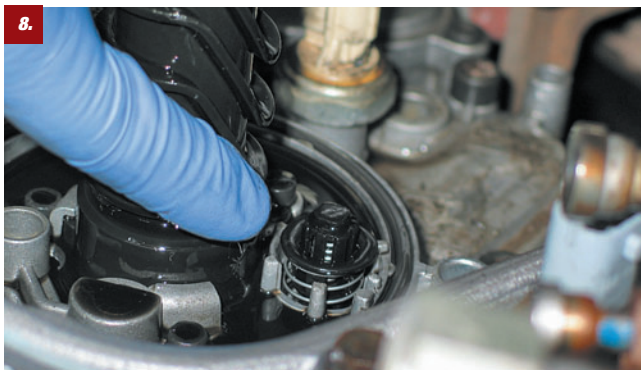
8. They also said this plastic drain-back valve has also been known to have problems. Since you are disassembling the engine, now is a good time to address these issues as well.
