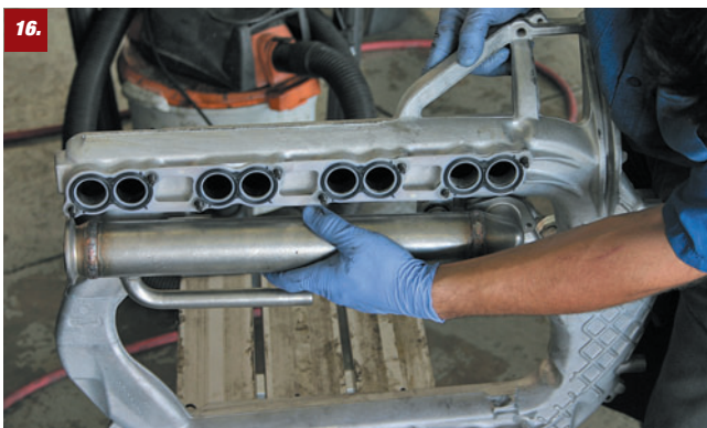
16. This shot illustrates the relationship of the EGR cooler under the intake manifold. Pictured is the new Bullet Proof Diesel EGR cooler.
