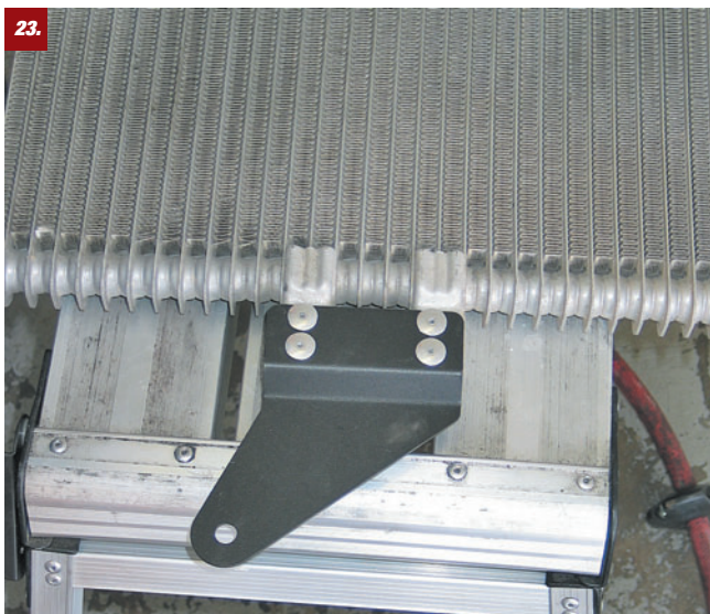
23. Here's a shot of the factory trans cooler with the new drop-down brackets attached.
