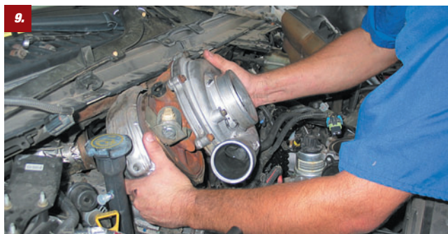
9. With the alternator out of the way, the stock turbo can be carefully removed. It's not as easy as it looks here.
