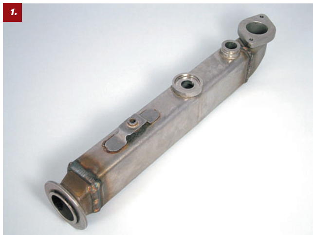
1. Bullet Proof Diesel's replacement EGR coolers are not only smog-legal, they also carry a lifetime warranty.
