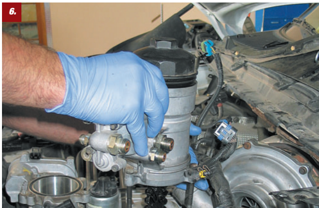
6. Once unbolted from the manifold, the stock oil-filter canister can be slipped off. Set it aside since it will be reused, sans filter, with the new oil manifold.
