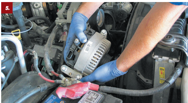
5. Access to the intake manifold requires removal of the alternator.
