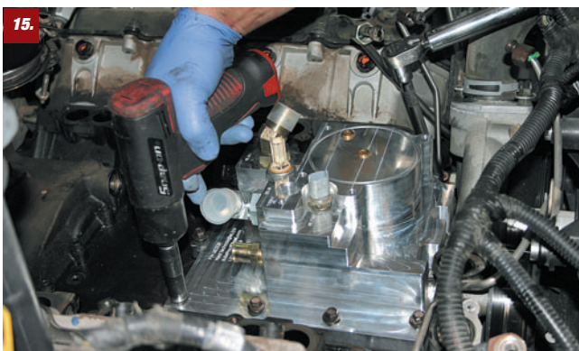
15. The Bullet Proof Diesel manifold assembly bolts in the stock location.
