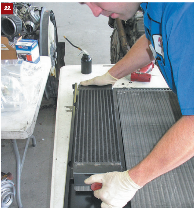
22. The ultra-heavy-duty oil cooler can now be positioned and mounted to the bracket.
