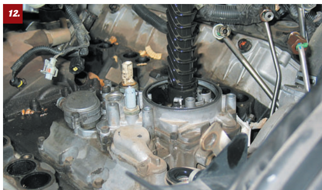
12. At the base of the oil-filter canister is this manifold assembly, which delivers both oil and coolant to the factory oil cooler underneath.
