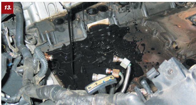
13. The factory oil cooler sits in this oil-filled trough just below the manifold assembly.
