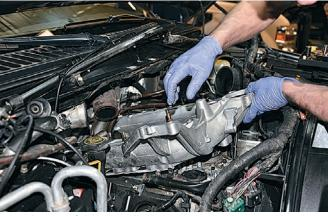
Next the manifold is installed.
