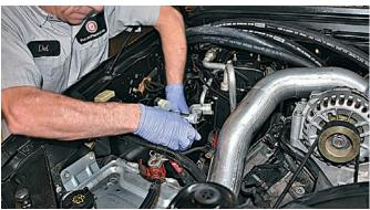
Del places the assembled oil cooler relocation plate and oil cooler into the new bracket and secures it with the provided hardware.
