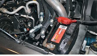
Each coolant and oil hose can now be connected to the proper fitting.
