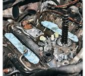
The old EGR cooler is replaced with Bullet Proof Diesel's proven replacement.
