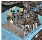
After cleaning the seal groove of the OE oil filter base, the provided replacement seal is added and then bolted to the new oil cooler transfer block.
