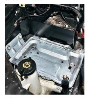
After removing the battery and tray on the passenger side, the black oil cooler bracket is installed after the vacuum reservoir is also removed. Then the stock trav is reinstalled and is now part of the bracket design.
