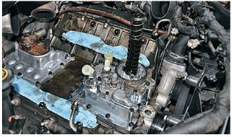
At this time the OE filter housing and oil filter are not reinstalled; this comes after the oil transfer hoses and intake manifold are installed. The old block will now be recycled since Bullet Proof Diesel recycles everything they possibly can.
