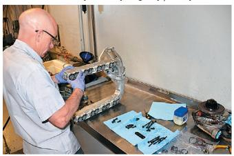
The manifolds are cleaned by a local radiator shop since they can clean them better than the in-house parts washer. Here Del Wamsley preps the manifold before he installs it. Every chance they get, BPD upgrades the hardware so no small part can possibly cause failure down the road. Again, it's the bulletproof theme the company is founded on.
