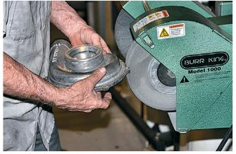
After assembling the turbo, Del puts the finishing touches to it by polishing it so it will really shine when the install is complete.
