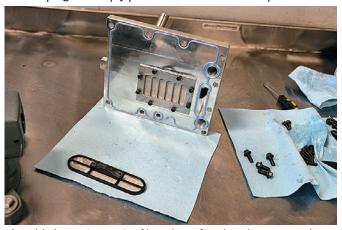
The old cheap OE HPOP filter that often breaks can now be discarded. You can see that the new BPD oil transfer block has an integral HPOP screen that is made from stainless steel and is a huge quality upgrade from the stock filter.
