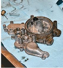
Following the OE oil cooler removal procedure—which included the removal of the intake manifold and turbo—Del removes the oil filter base that will be reused.
