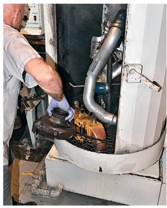
Extra steps are taken to give each customer the best possible service. First Del pressure washes the turbo housing, followed by a trip to have it sand blasted.
