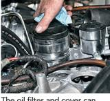
The oil filter and cover can now be reinstalled after all the hoses have been connected.
