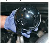
To make room for the new oil cooler, the old vacuum reservoir had to be removed. A smaller vacuum reservoir is provided and is easily installed on the side of the engine compartment.
