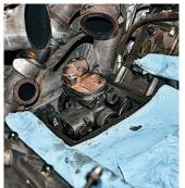
When re-installing the HPOP that is in the very back of the engine compartment, be sure to remove all of the oil and debris from the HPOP reservoir first.
