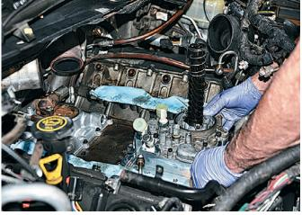
Using the OE bolts and following torque specifications, the new BPD oil transfer block can now be re-installed. The only downside to this polished piece is that it's now going to be buried where it won't be easily seen.
