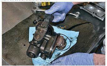
The upgraded high pressure oil pump (HPOP) pressure fitting replaces the original "snap-to-connect" fitting. It's a good idea while this is apart to do the optional STC upgrade.
