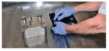
Using the OEM oil cooler hardware from the oil cooler removed earlier, the next step is to bolt the new oil cooler to the relocation plate.
