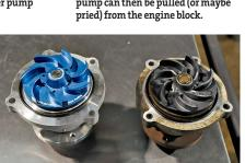
finish of the aluminum impeller once installed, you'll have to be content just knowing that it's stiffer, stronger, and won't crack along the hub.
