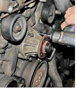
With everything finally out of the away, there are only four bolts to be removed and the water pump can then be pulled (or maybe pried) from the engine block. Assuming that your radiator is good, your head gaskets aren't blown, and there are no leaks that cause you to lose coolant, your overheating issue is likely a broken or cracked water-pump impeller. It's impossible to tell if the plastic impeller is damaged unless you remove it from the engine. This one was toasted.
