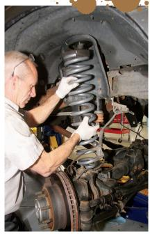
With the four-link arms installed, the front axle was lowered until the taller Rough Country coils could be slipped into place. Different rate coils are provided, depending on whether the truck is a gas or diesel model.
