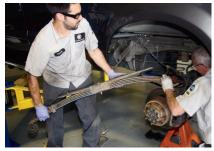
11 With the front four-link complete, the team turned their attention to the rear suspension. The aged shocks and factory leaf packs were pulled off to make way for Rough Country replacements.
