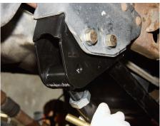
Here you can see one of the control arm brackets that attaches to the factory frame mount, moving the link mounts downward to keep the radius arms flatter with the added lift. This eats up a little ground clearance under the frame but retains good suspension geometry for better handling.
