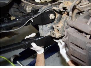
The upper and lower radius arms are made from heavy wall tube and the axle ends are heavily boxed with plate. These mount in place of the factory swing arm-style radius arms.
