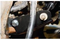
A plate mount is provided to drop the steering stabilizer downward, and steel brake line relocation brackets allow reuse of the factory lines. The front ABS wiring was moved slightly and secured with tie-wraps.
