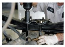
12 The factory shackles were mounted onto the new leaf packs. The basic kit comes with add-a-leaves and blocks, but the truck owner opted for the complete replacement lift packs. These offer improved ride and better flex over using the old packs.
