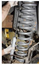
was jacked back up to near ride height and the factory track bar was bolted into the new drop bracket.
