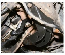
The guys started by removing the steering linkage from the pitman arm, disconnecting the sway bar end links, and disconnecting the stock track bar. A new dropped pitman is included in the kit, and a dropped bracket for the track bar moves the attachment point downward to help preserve proper front suspension geometry.
